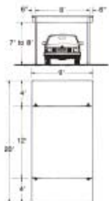
HALF BAY WITH OVERHANG ROOF
